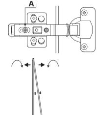
Adjusting the angle of the door. Loosen screw 'A' and slide the hinge arm either forwards or backwards until the door is vertical then tighten screw 'A'.
