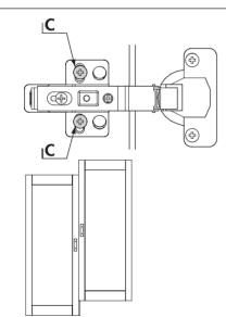
Adjusting the height of the doors. Loosen screws 'C' then slide the hingeplates up or down until the doors are even then tighten the screws.
