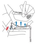
8.Pull the base separation handle, and lift up the handle of the carrier to separate the carrier from the ISOFIX base.
