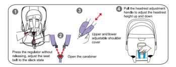
Tips: Make sure that the height of the seat belt is at the same level as the child's shoulder height or slightly higher than the child's shoulder height.
